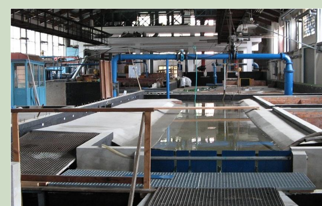
Physical model (hydraulic laboratory at WRI) – crossing of the Čiliž brook and canal – inverted siphon design & flow regime optimization
